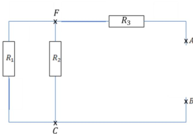
$$R_{Th} = \frac{R_1 R_2}{R_1 + R_2} + R_3$$
